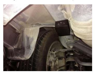
Note: If the tracker has not been attached to the vehicle for over 5 seconds, a drop alarm will be generated. After 5 minutes, if no event (incoming call/SMS/vibration) is triggered, the device automatically enters the deep sleep mode. In any mode, the deep sleep mode will be automatically enabled after the drop alarm is generated.
